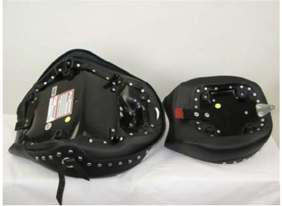
2. Lift the passenger seat and handstrap off the motorcycle.
