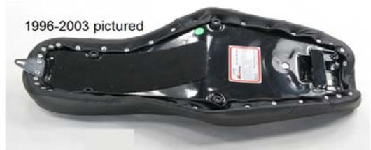
2. If one-piece, slide the seat up and back to disengage the front bracket and remove the seat.
