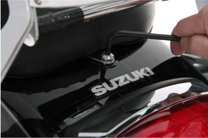
5. Position the black  $\frac{1}{8}$ " nylon washer between the rear bracket and the fender, and secure to the fender with the stock 8mm rear bolt and metal washer.
