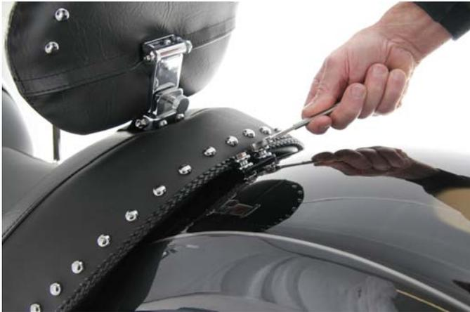
3. Position the passenger seat on the fender and slide it forward until the front forked bracket engages the spool washers.
