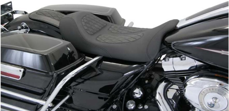
5. Once the solo is in position, slide it back as much as possible so the baseplate firmly and tightly engages the mounting nut.
